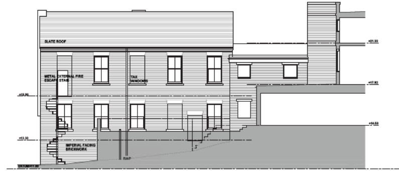
2 SOUTH-EAST ELEVATION (3 CONEY STREET) 1:100
